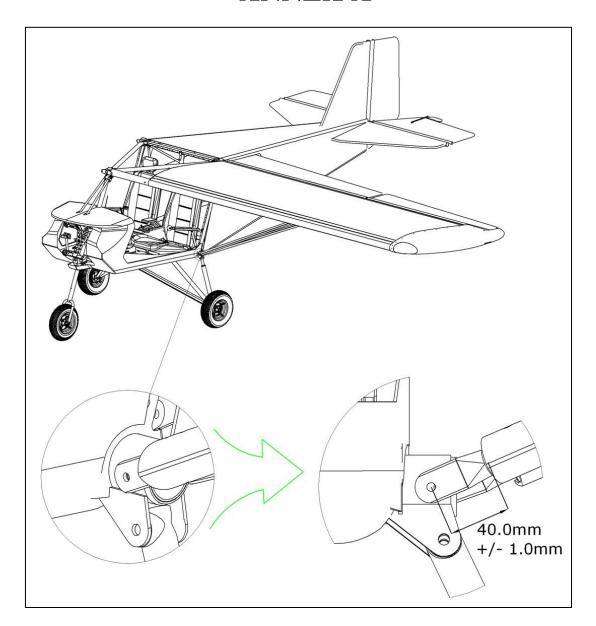
Note: Measure the distance from the centre of the Front wing strut mounting bolt to the edge of the wing strut. The distance should be 40.0 mm +/- 1.0 mm.
