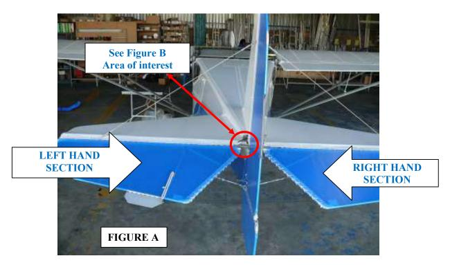
Due to the amount of flight hours accumulated on this aircraft it was found that this tie point has cracked off because of fatigue.
