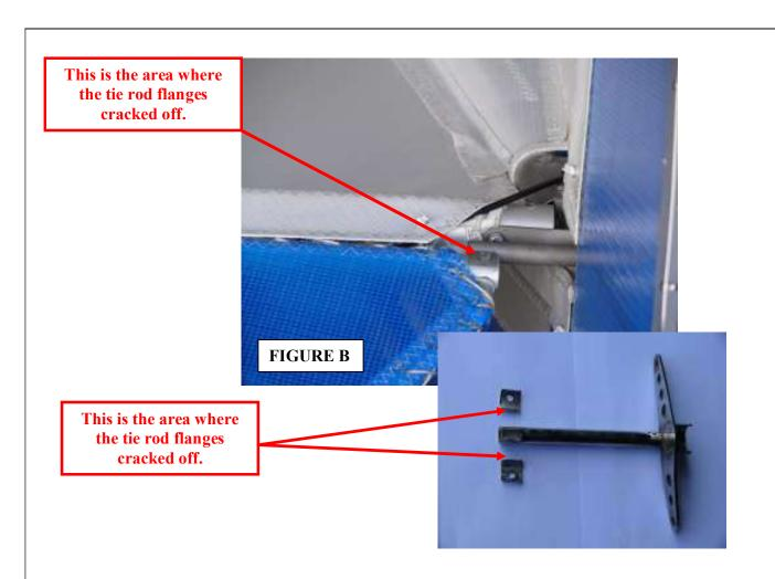
This tie rod needs to be replaced with a newly designed tie rod as shown in figure C as indicated in paragraph 1d.
