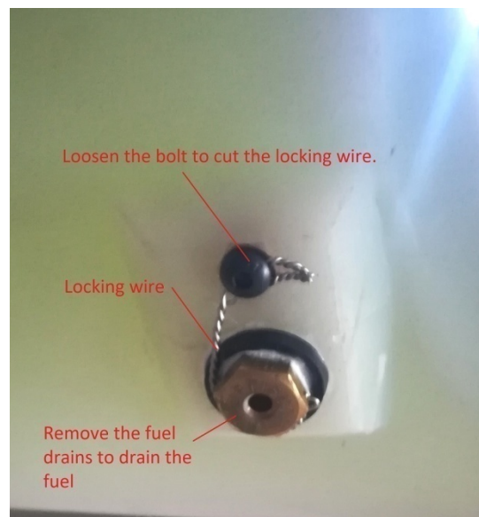
Figure 1: Fuel drain at the bottom of the tank
