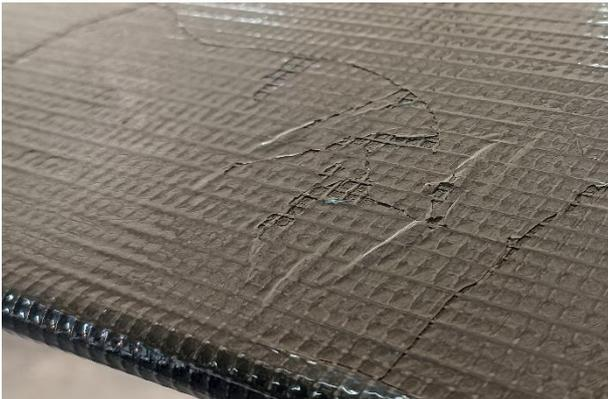
Figure 1: Example of Delamination and Cracking of an Aileron Sail
