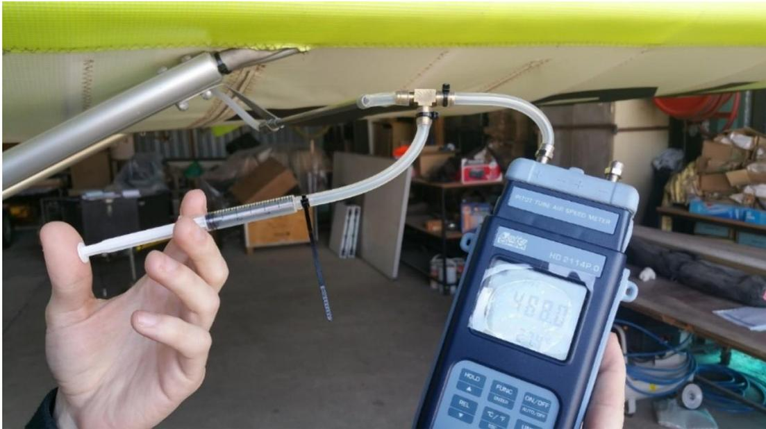
Figure 1 Arrangement of instrument calibration system
