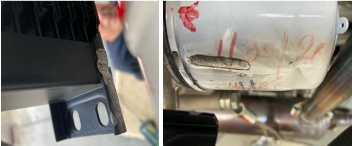
Figure 2 – Lower oil radiator and oil filter housing
