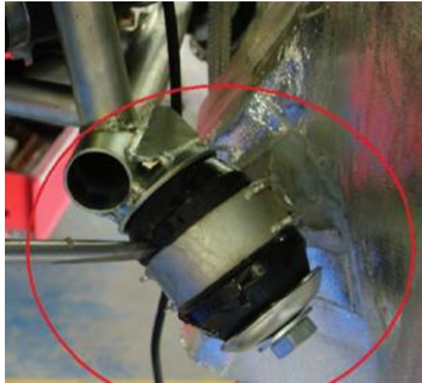
Figure 5 – Correct mount rod
