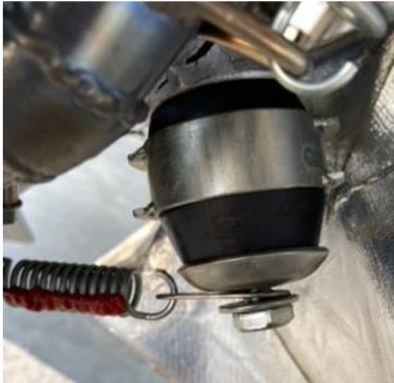
Figure 4 – Defective mount rod
