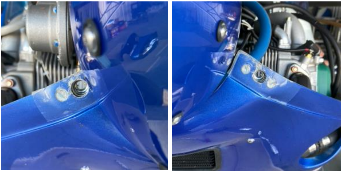
Figure 1 – Engine shifted to the right
