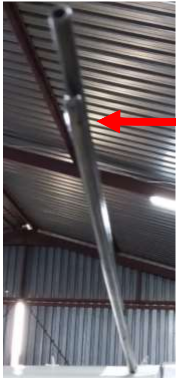
Figure 1: Location of static ports (on lower tube)
