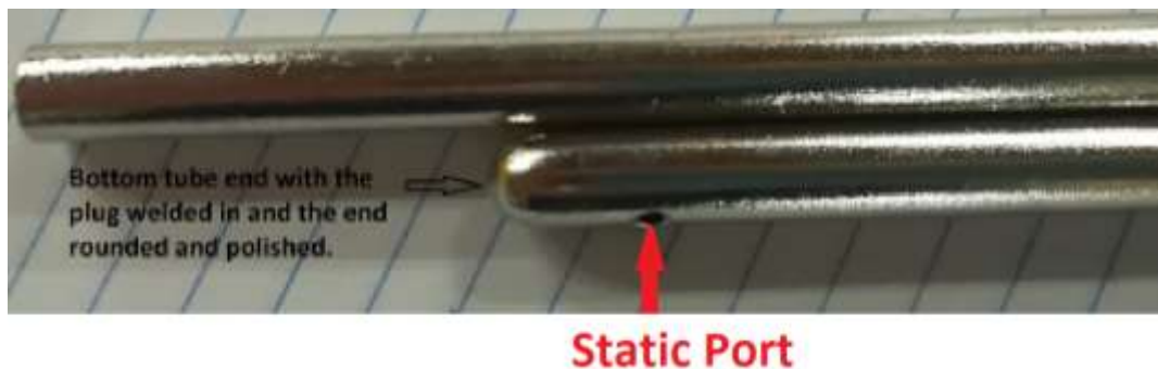
Figure 2: Close-up of static port (one visible, not installed on aircraft)
