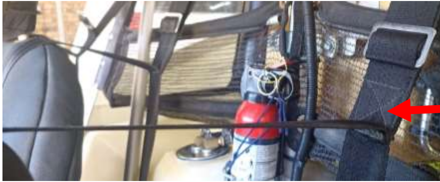
Figure 1: Belt Pulled Horizontal by Seat being pushed Forward (Stitching area to inspect shown by red arrow)
