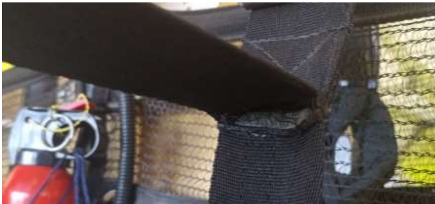
Figure 3: Belt Separation Visible from Below
